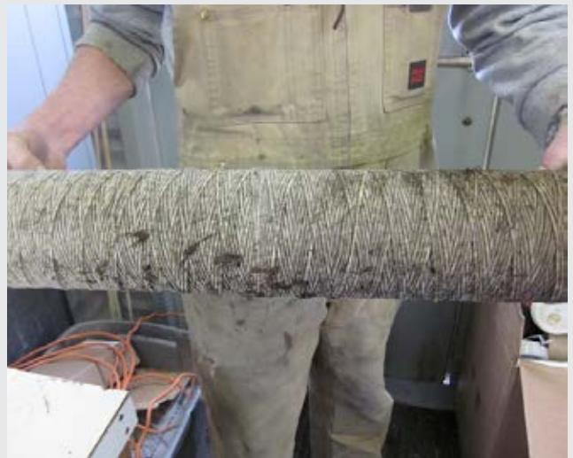
An operator displays a used filter. Filtration is a relatively recent addition to this small town's water supply.
